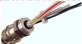
**b)** Position the SST Wire Sleeves so they are .5" inches from cable jacket and the cartridge is centered between them. Crimp SST Wire Sleeve to central wire using .128" die.
